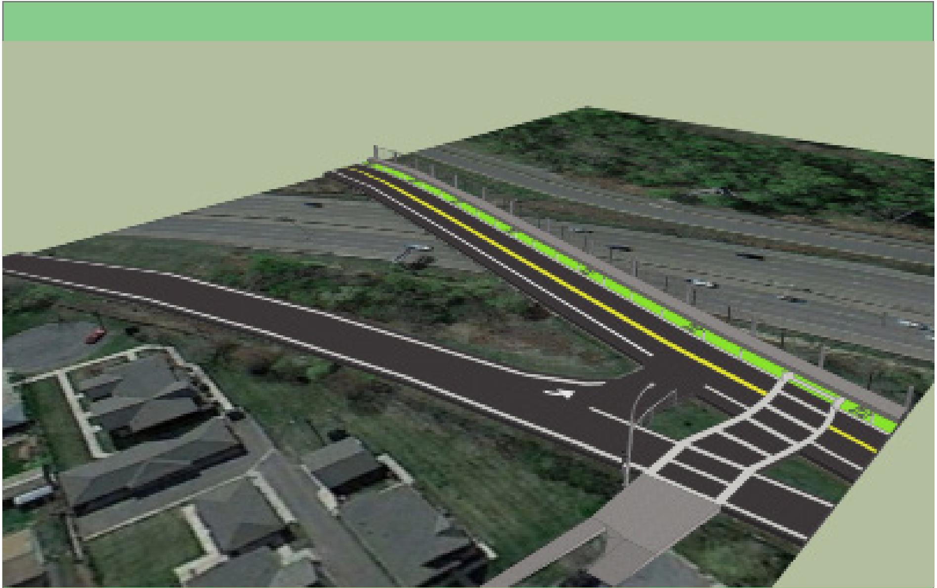
Above: A rendering showing the proposed crossing from Surrey Avenue (at bottom) across Mounds Boulevard, with additional improvements over the Mounds Boulevard bridge. Note the zebra striped crosswalk, the overhead pedestrian warning signal for cars, and the bike lane along Mounds Boulevard.
