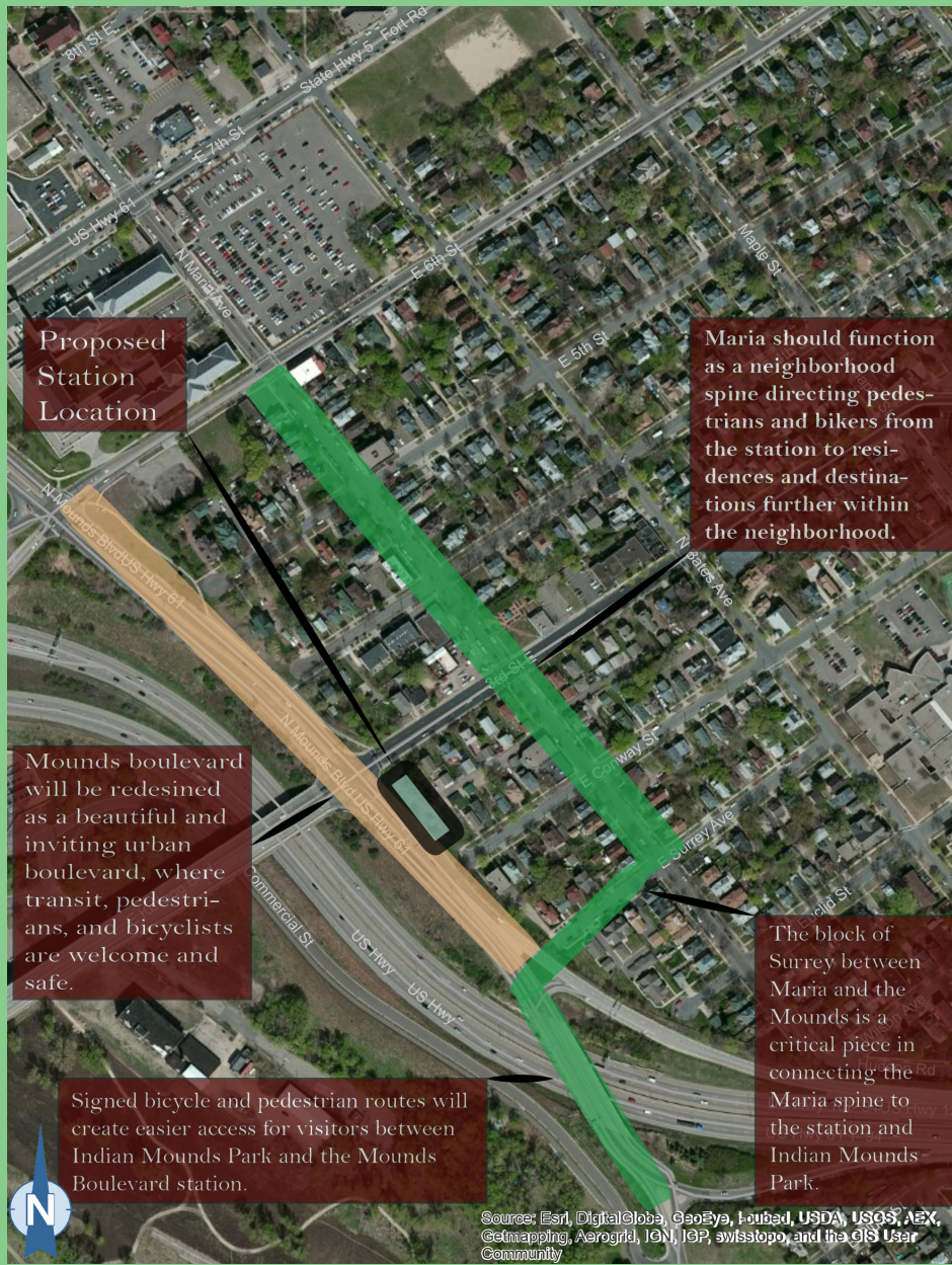
Overview of treatments to proposed station area. Green: Pedestrian and bikeway connections. Tan: Road and intersection diet.
